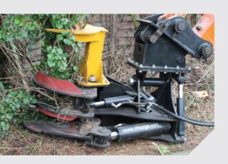
The Scorpion 440 is an excavator mounted tree shearing and removal device aimed at reducing the time and labour overhead on tree removal and de-limbing operations. Ideal for controlled sites such as road side works.
